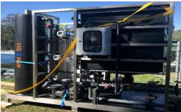
The ultrafiltration system will have two uses: (1) to clean the brackish river water to remove all microorganisms including viruses before it is used in the algae ponds; and (2) during harvesting to pre-concentrate the algae-laden pond water 20-fold prior to flowing into the centrifuge for final concentration into a dense paste. During harvesting, the clean ultra-filtered water is temporarily stored until it is recycled to the pond to allow growth of algae to resume.
