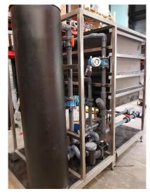
The small ultrafiltration system continues to be assembled by our supplier in the Netherlands. The latest photograph provided (at left) shows the frame and the filtrate tank installed together with two pumps. The control panel and the filtration modules will be installed in February with shipment to Qponics expected at the end of that month. A large specialised algae centrifuge is expected to be purchased and installed in February.
